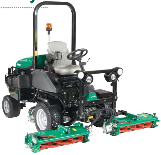
Specifically designed for the commercial market, the Highway 3™ triple cylinder mower is compact for easy transport, with a high specification and low weight. The Highway 3™ triple cylinder mower is significantly lighter than its predecessor, highly manoeuvrable, easy to maintain and is an ergonomic delight for operators.
